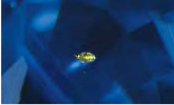
This unheated sapphire from the Ban Huai Sai area, Laos, contains a conspicuous inclusion of yellow monazite. Photomicrograph by S. Singbamroong, ©Dubai Gemstone Laboratory; magnified 25×, oblique illumination.
